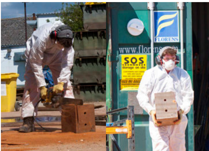
Safety first (No Time To Lose): Projects' Joe Funnell wore a dust mask, impacted goggles and a paper suit when cutting timber
