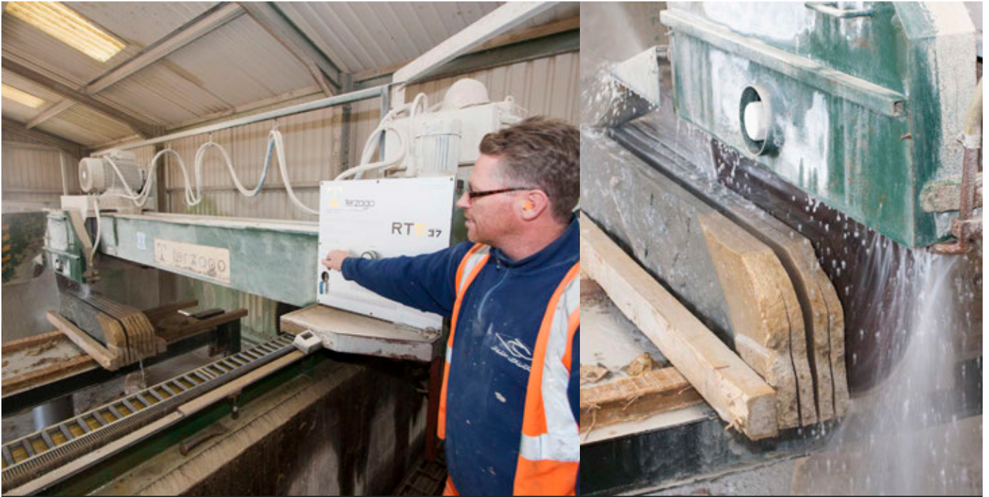
Chip off the old block: (left) Mark Cockwell carried out primary sawing with a Terzago RTS37 bridge saw (right)
